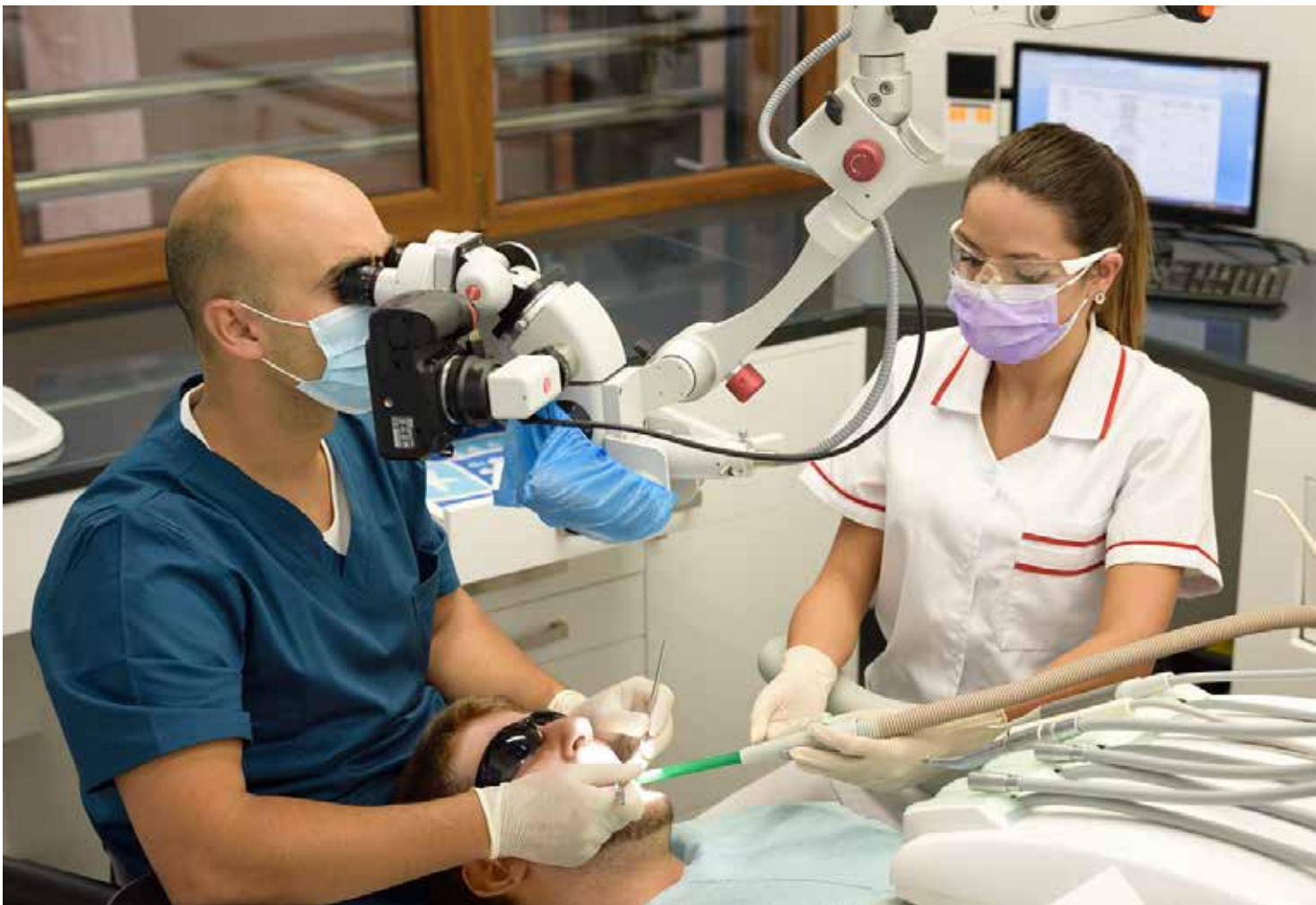
For an ergonomically correct working position - Kaps 1100 with 45° ergonomic wedge with beam splitter, binocular turntable and photo tube (Image with kind permission of Dr. Milen Dimitrov)
